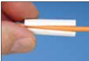
Apply LABELCORE™ sleeve to cable
